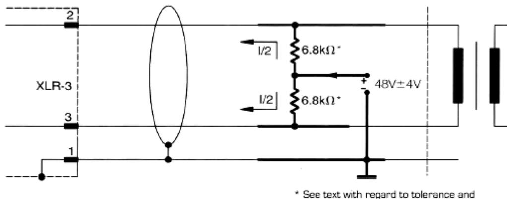
*Figure 1 - A standard 48 Volt phantom powering arrangement
