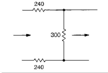
*Figure 4 - Balanced resistive pad, suitable for use with phantom-powered microphones*
