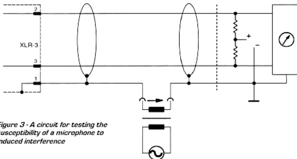
*Figure 3 - A circuit for testing the susceptibility of a microphone to induced interference*
